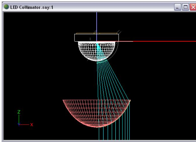
The central lens is now drawn and ready to be integrated into the rest of the collimator, which we can now continue to create. Next, we will create the complete hemispherical entrance.
