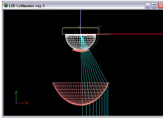
The collimator entrance is currently only within the angular sweep of the central lens. In order to use a complete hemispherical entrance, we will need to redraw a separate piece of geometry. However, if this smaller piece of entrance also remains, there will be an error in the way our collimator is drawn and it will not calculate correctly. We can make this smaller piece of entrance surface inactive to avoid this problem.
