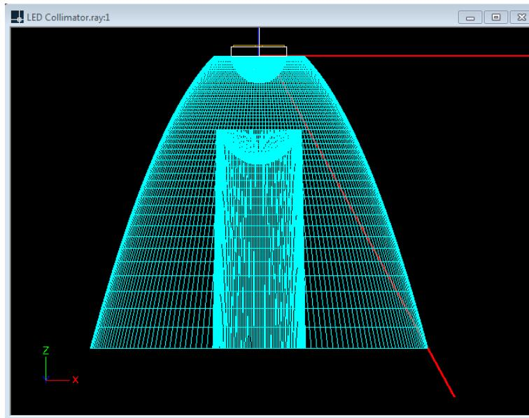
35. Use the line command again to draw a line from 2.5,0 (the start of the TIR profile) to 2.5,-20 (a point directly below the start point). This is the boundary line for light reflecting from the TIR surface, meaning that if part of the center lens or shaft is to the right of this line, that part will
