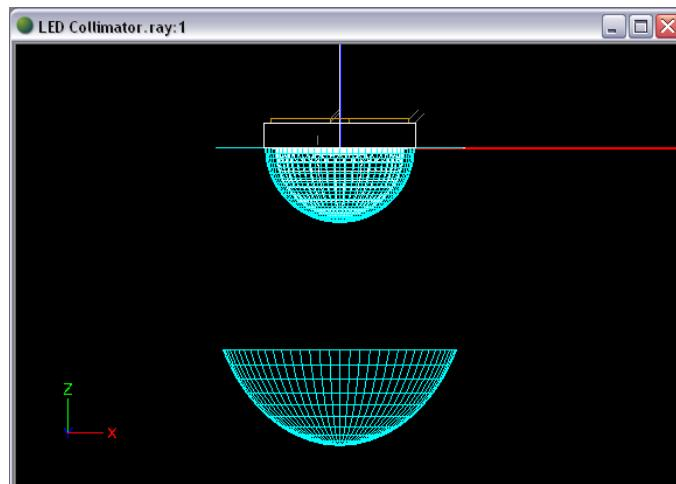
18. You can ensure that the surface is oriented correctly, as shown below, by right clicking in CAD view and choosing **View Style > Show Surface Orientation**, and then using orbit. You can then return to the original view style by selecting **Wireframe**.
