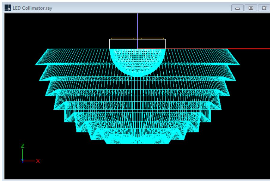
A lens has been generated as you can see in the CAD view, but we still need to make a few adjustments to get to the smooth convex central lens exit for the collimator.
