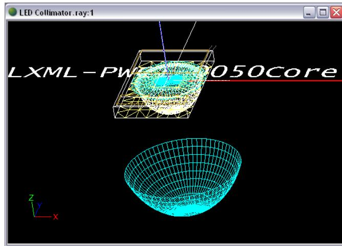
The new refractor segment will be hard to see, but if you orbit in CAD view you should be able to find its cyan lines. To turn the new refractor segment into a revolved arc:
