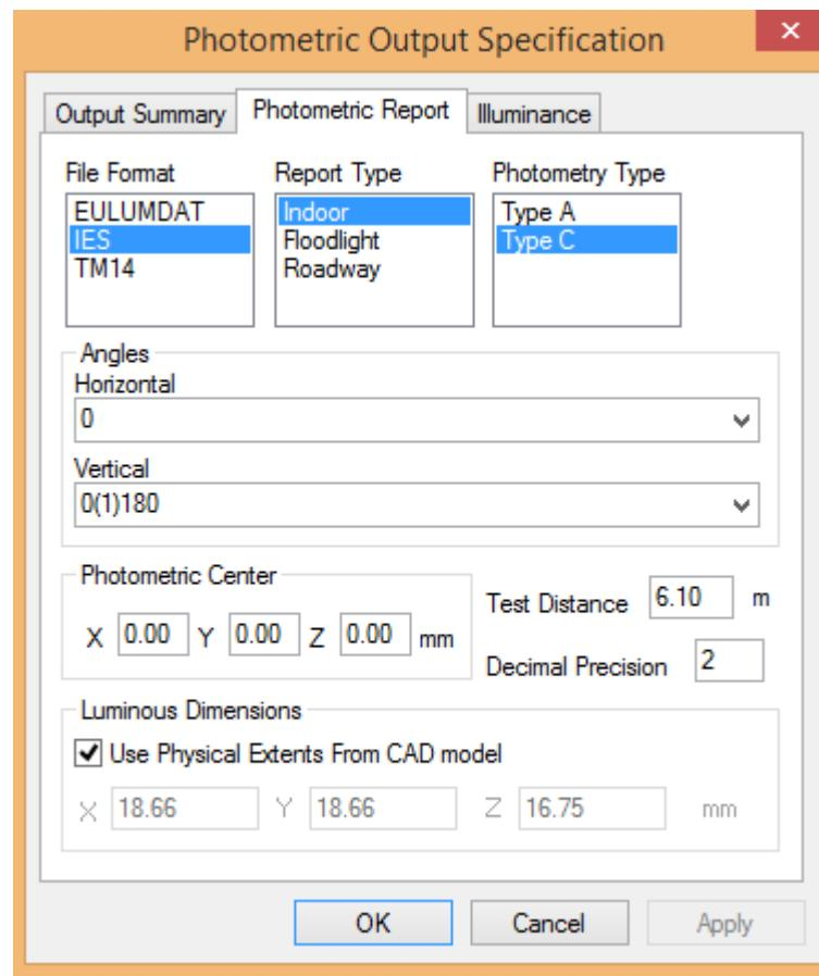
41. Under the Illuminance tab of Photometric Output Specification, create an illuminance plane 1m x 1m, 1m below the collimator. Click OK in both the Illuminance Plane window and the Photometric Output Specification window.
