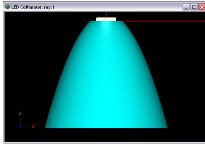
Next, we can link the TIR surface profile to the base surface profile. Again, even though we constructed the TIR profile to start where the base profile ended, if you later decide to change the diameter of the entrance or the base (for example, if a different size LED is to be substituted into this design), the TIR surface will automatically adjust if we link it to the base surface.
