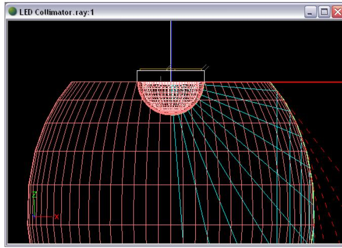
This central lens cannot control the entire distribution, as you can see by the red dashed warning lines that indicate the desired refraction is not possible there. For this reason, we will end up using a TIR surface to control the higher angle light. The central lens should control the light from nadir up to about 30°, so we need to adjust its angular sweep.
