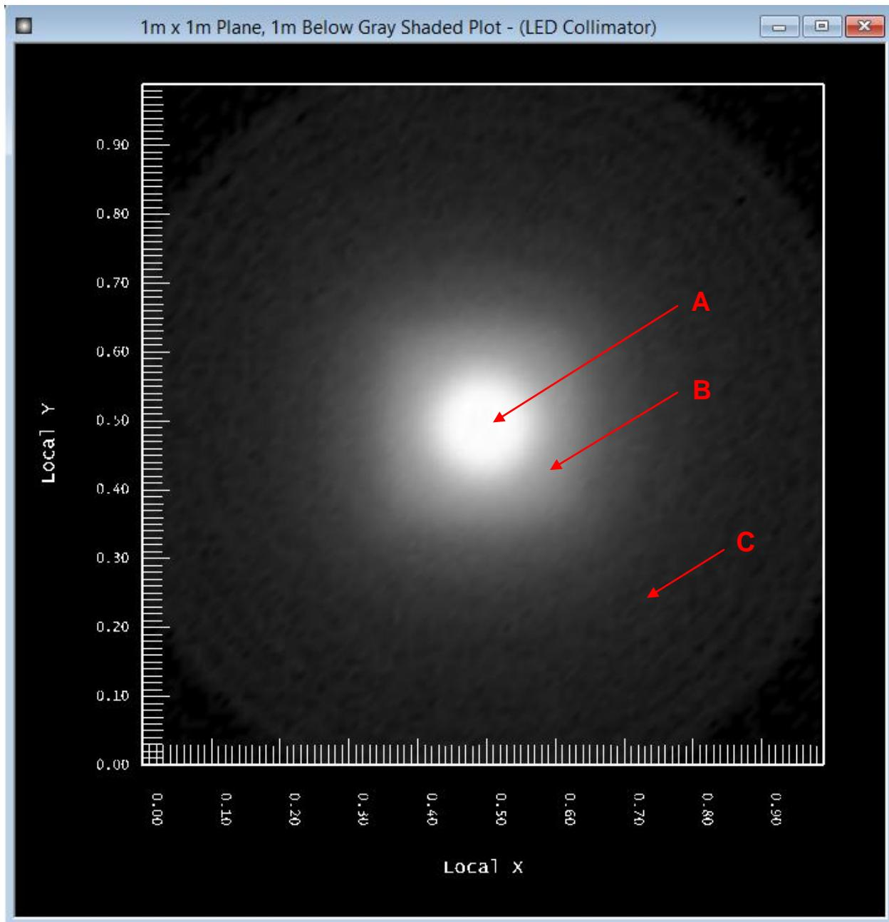
The spot labeled 'A' is the resulting pattern from the TIR part of the collimator. The spot labeled 'B' is the resulting pattern from the central refractive lens part of the collimator. The spill light labeled 'C' is an unintentional side effect of interactions between lens surfaces.
