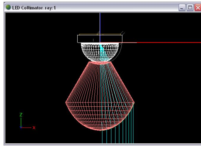
The central lens is now starting to take the expected shape. There are still a couple of adjustments to help integrate this lens with the rest of the collimator.
