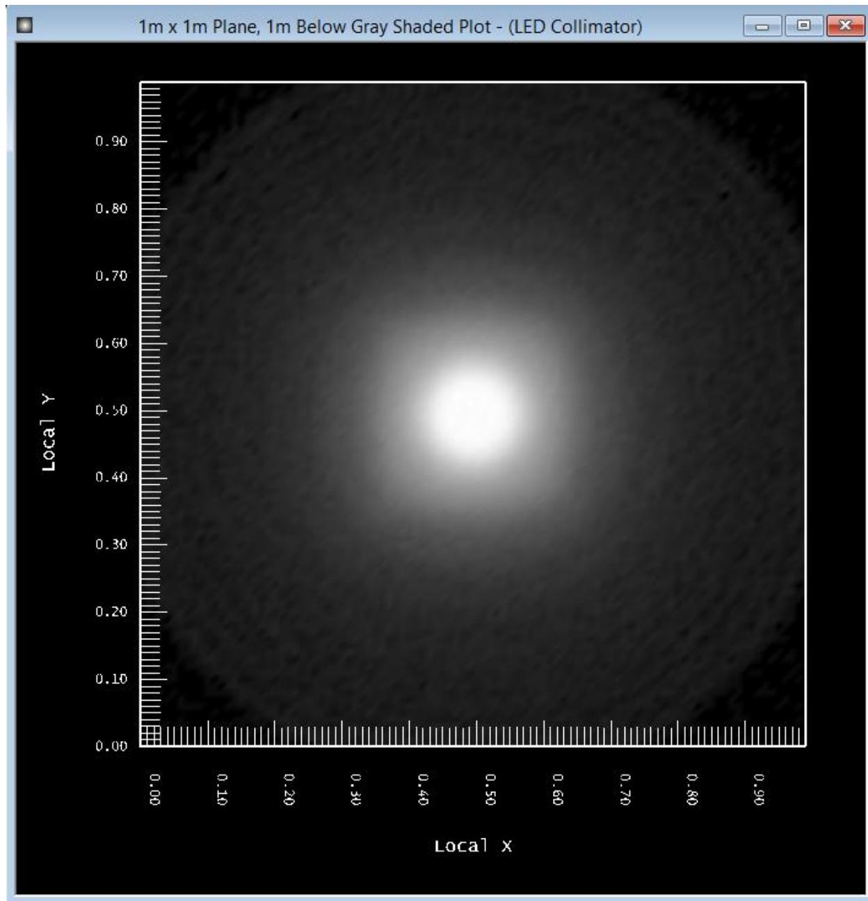
The full beam angle is within  $1^\circ$  of the beam angle goal of  $10^\circ$ , the illuminance pattern looks decent, and all the design parameters have been met. The design and material of the collimator also produces an optical efficiency in the high 90's, as can be seen in the Photometric Report, but note that a housing has not been included in the model yet.
