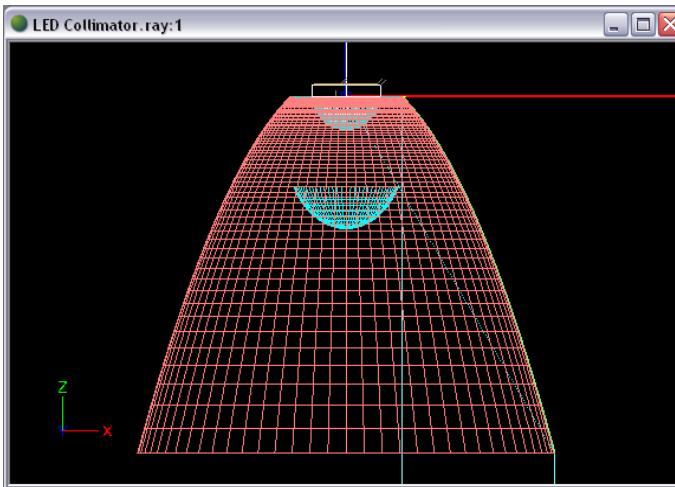
The TIR surface is automatically oriented toward the lamp center, as you can see by right clicking in CAD view and choosing **View Style > Show Surface Orientation**. In this case, that orientation is incorrect since it is the outer surface of a lens. Refractor surfaces should always enclose a 3D space and be oriented outward from that space.
