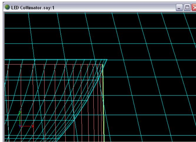
32. In Parametric Optical Design View, adjust the Length values of both sections of the exit surface in order to make it more precisely meet the end of the central lens profile. Using Lengths of 6.77 mm for the Start section and 12.08 mm for the End section creates a precise intersection.
