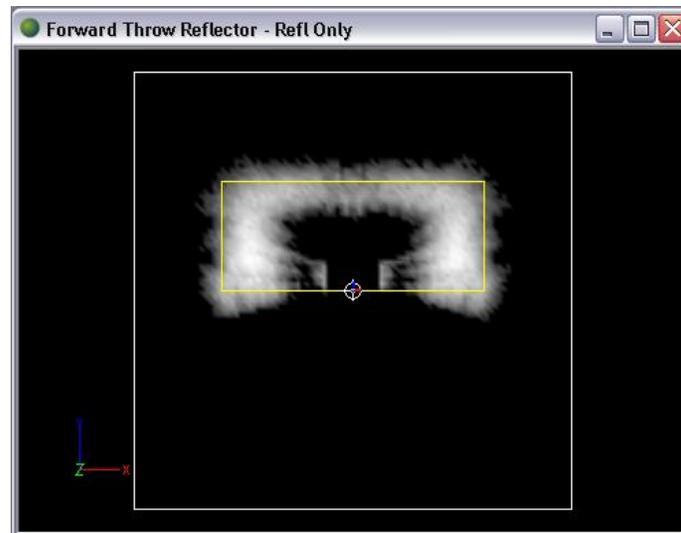
Now we can see that almost all of the light is enclosed in the target area, and there is an open area in which the direct light will fill in. Thus, the isolated reflector itself does a good job at controlling the light to obtain the desired results.
