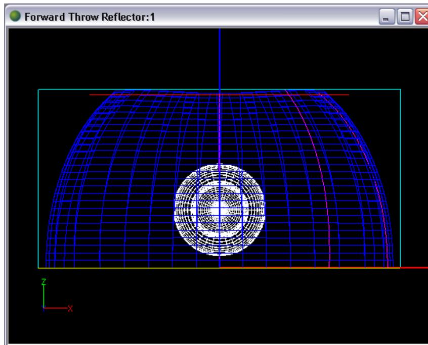
70. Create a new layer for top reflector, naming it *REFL-Top Reflector* and giving it a color such as red. In CAD view, click on it and change it to the appropriate layer.
