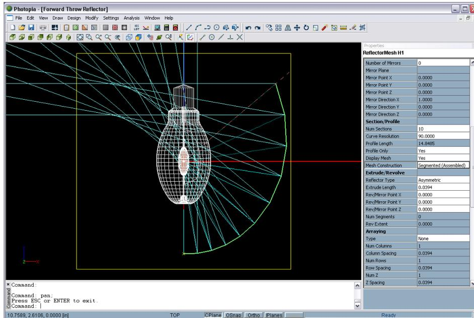
12. To create the first vertical profile, first go into left side view, and ensure that the CPlane is set to the current view. We will create the first vertical profile at the center of the back of the optic, so in this view it will be to the right of the lamp.
