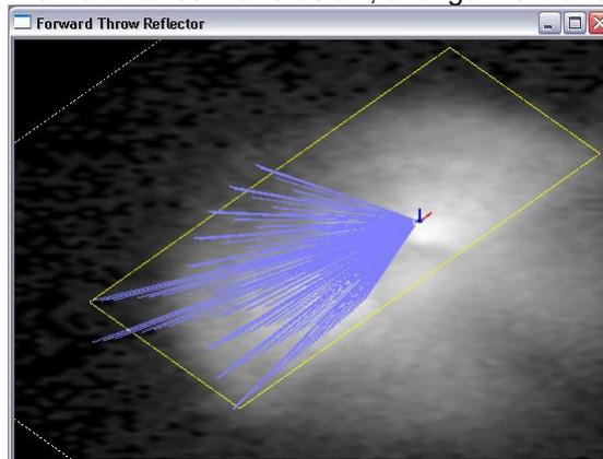
By orbiting in CAD view, we can see that the new V2 profile will better reach the corner of the target area. From this view, it also looks like we might want to slightly raise the aiming angles of V3.
