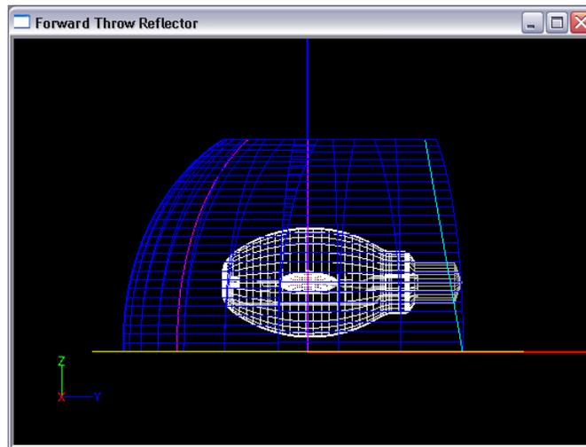
32. Linking the front reflector to the main reflector will make the position of the front reflector adjust automatically when we make changes to the main reflector. Select the front reflector and under **Start & Extent** in the property control change the Start Linkage from *None* to *H1*.
