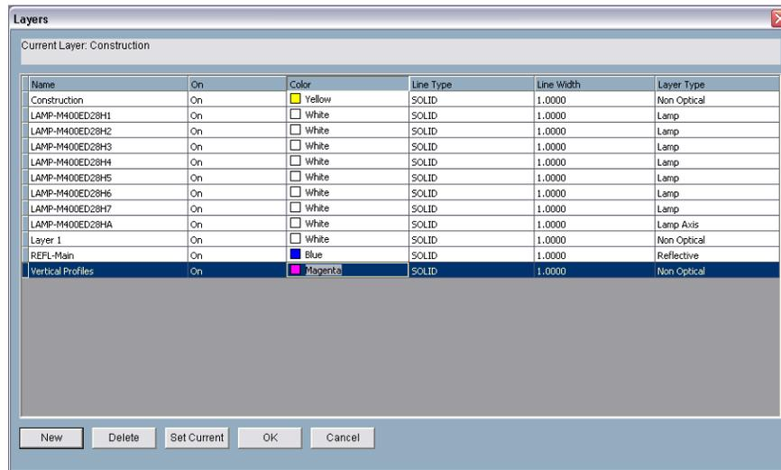
22. Select the vertical profiles and change the Layer in the property control to the appropriate layer name.
