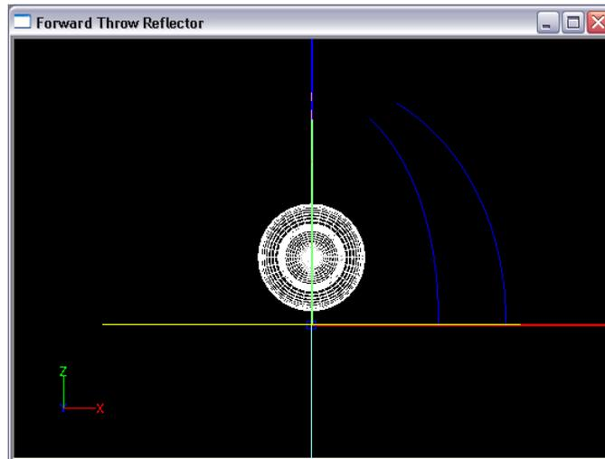
You can see from this view that changing the start point of V3 had a secondary effect of making it taller. The height of the profiles is based on a reflector extent angle rather than a fixed height, so we will need to adjust this angle to bring V3 back to the same height as V1 and V2.
