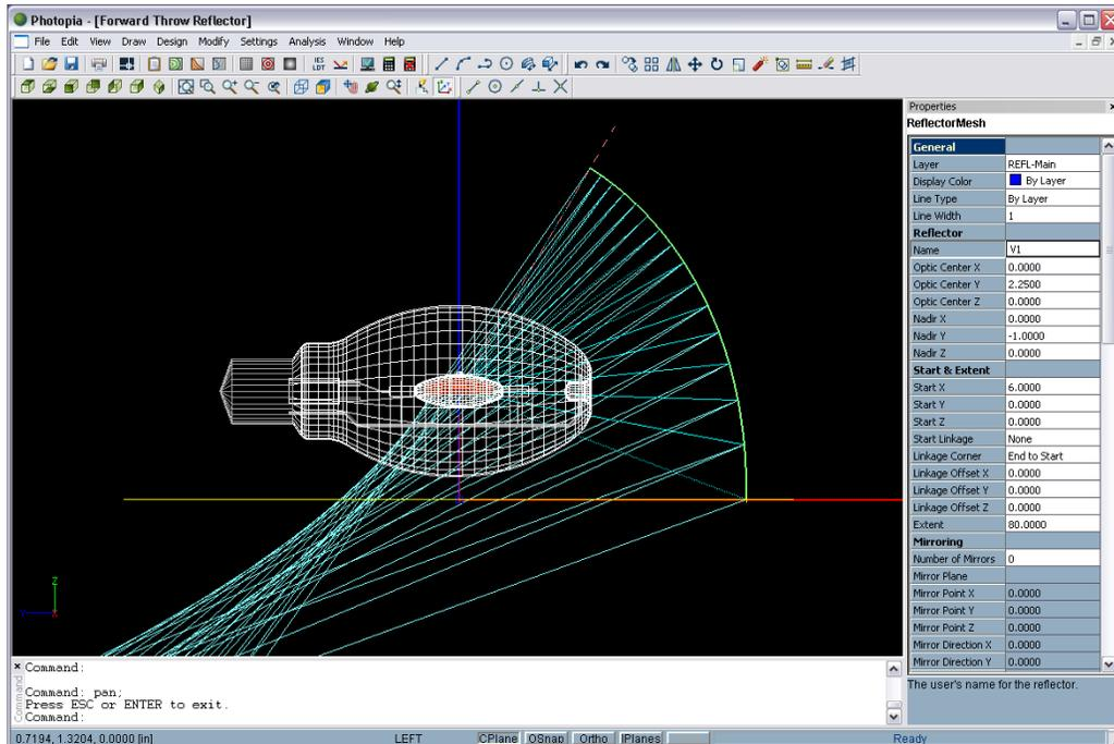
15. Next, we will array copies of *V1* so that we can have multiple vertical profiles. We will then be able to adjust the profiles individually, and so the optic's vertical profile will differ depending on where it is on the horizontal profile. From top view, choose **Modify > Array** from the main menu to run a polar array on profile *V1*.
