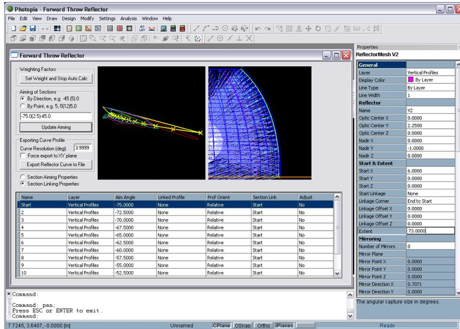
47. To view where the light is aimed to hit the Illuminance Plane, we can use the **Aiming Lines** section in the property control. Find it near the bottom, while H1 is selected from top view. First change the Aiming Display from *Off* to *On*. Update the Effective Lamp Point Z to 2.25. To get the aiming lines to reach the Illuminance Plane below, change the Plane Point Z to -240.
