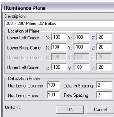
39. In the CAD view, click on the Illuminance Plane to change Display Plot under **Display** in the property control from *False* to *True*.
