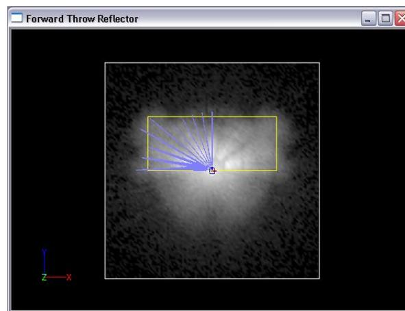
The corner light has filled in well, but there are still bright spots near the center of the light pattern. To continue working on this issue, we can adjust the weighting of the other vertical profiles as well.
