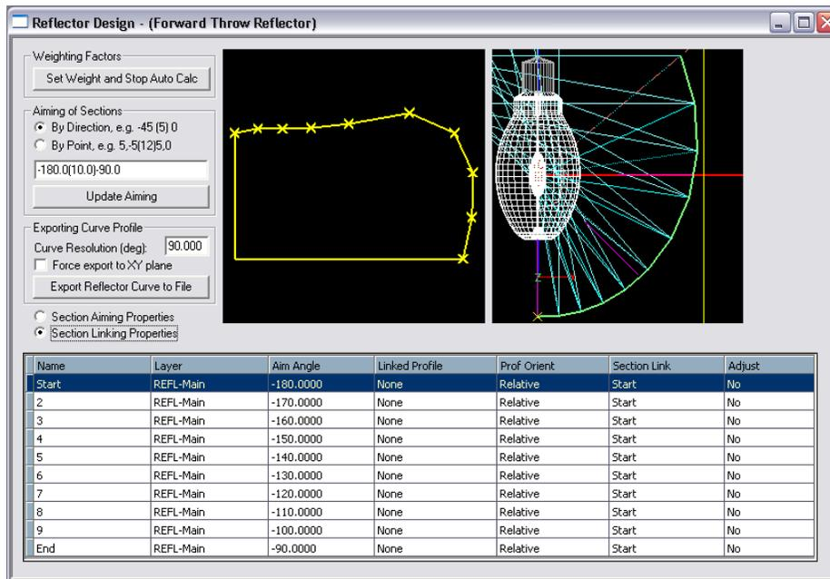
We will use V1 for the front of the light pattern, V2 for the corners, and V3 for the sides. To do so, we need to assign each vertical profile to particular sections of H1.
