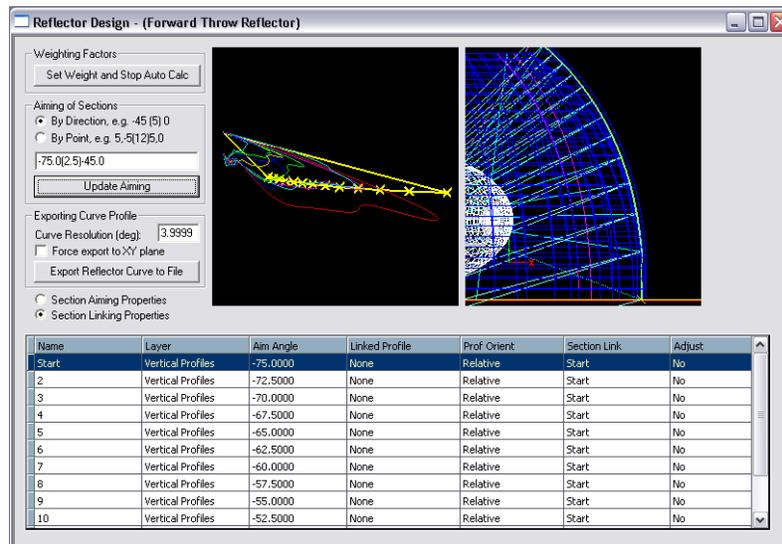
45. Adjust the aiming weighting of V2 by changing the Weight Exponent under **Weighting** from 1 to 2. You can see the yellow aiming diagram in Parametric Optical Design View update with heavier weighting on the higher angles.
