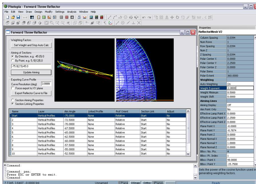
46. Adjusting these factors of V2's shape has caused it to become taller than the other vertical profiles, as previously discussed. Change the Extent under **Start & Extent** to  $73^\circ$  for a height that better matches the other vertical profiles.
