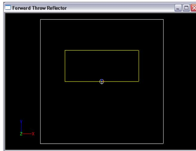
41. From front view, move the target rectangle down 239" so that it is just above the Illuminance Plane.
